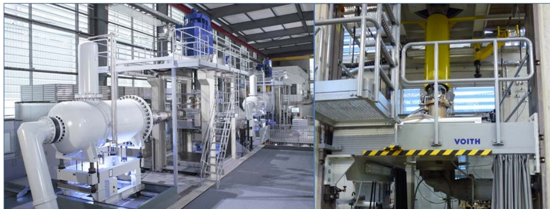
Figure 10: Universal High Pressure Test rig at the “Brunnenmühle” hydraulic laboratory in Heidenheim (left). With the Veytaux II model machine mounted (right).
